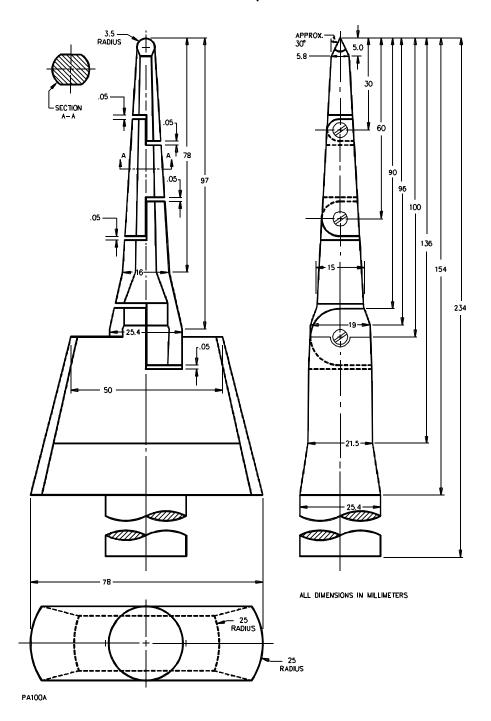
Figure 6.2 Probe for film-coated wire
