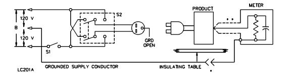
$B-240\ \text{or}\ 208\ \text{volt}$  product intended for connection to 3 wire grounded neutral power supply.
