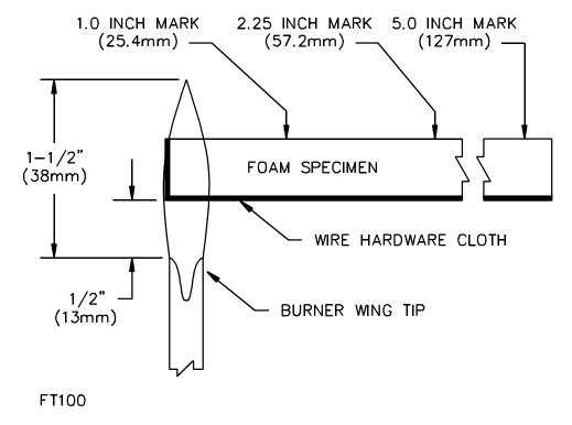
63.4.7 The flame is to be applied for 60 seconds and then removed from the specimen. If the material continues to burn after removal of the test flame, the time for the flame to travel from the 1 inch (25.4 mm) mark to the 5 inch (127 mm) mark is to be determined. If the specimen ceases to burn before the 5 inch mark is reached, the duration of burning after removal of the test flame and the distance of burning from the end exposed to the test flame are to be recorded.
