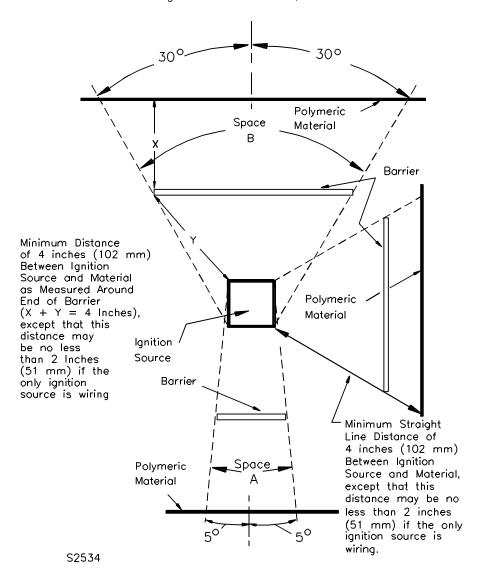
Space A – Represents the volume below the ignition source determined by a straight line that moves about the ignition source while remaining at an angle of 5E from the vertical and is always so oriented that the volume is maximum.
