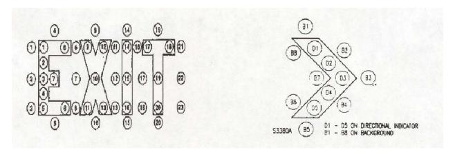
The luminance for each numbered position in the legend and directional indicator shall be measured over a circular area as large as possible while maintaining at least a 1.6 mm distance between the perimeter of the circular area and the adjacent border. The positions for measuring the luminances of the background shall lie within 25.4 mm of the legend and directional indicator but no closer than 1.6 mm to the border.
