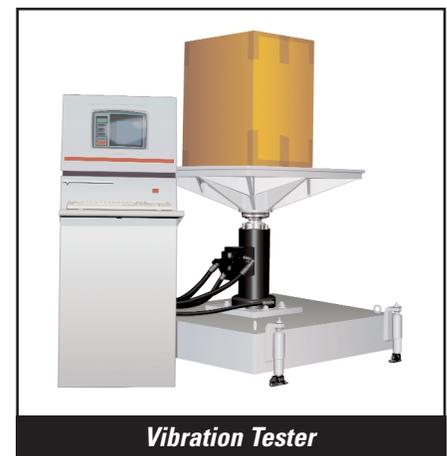
NOTE: FOR INTERNATIONAL SHIPMENTS, A SECOND SERIES OF DROP TESTS WILL BE PERFORMED FOLLOWING THE VIBRATION TEST.
