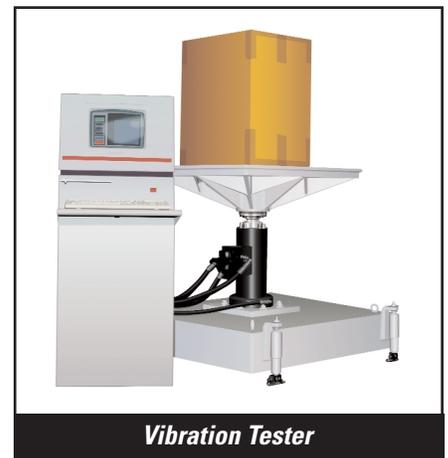
\*\*\* Current vibration system can test packages up to max. 200 lb. Contact FedEx Packaging Design and Development before sending test packages over 200 lb.
