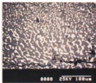
Figure 2. SEM microstructure of a thermally fatigued Sn63/Pb37 solder joint, showing the coarsened area near the interface.
