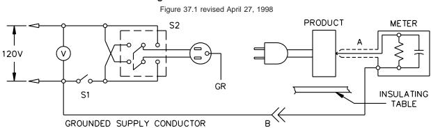
Figure 37.1 Leakage current measurement circuits
