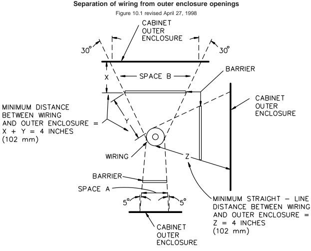
Figure 10.1 Separation of wiring from outer enclosure openings
