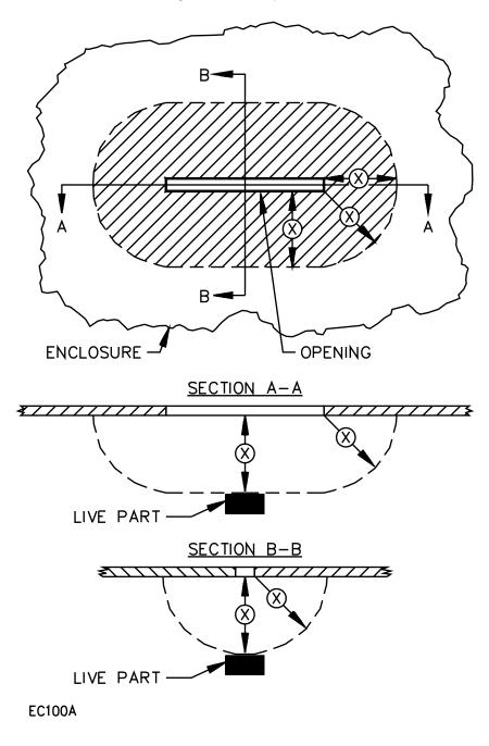
The opening is acceptable if, within the enclosure, there is no uninsulated live part or film-coated insulated wire (1) less than X inches (mm) from the perimeter of the opening, as well as (2) within the volume generated by projecting the perimeter X inches (mm) normal to its plane. X equals five times the diameter of the largest diameter rod which can be inserted through the opening, but not less than 4 inches (102 mm).
