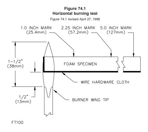
74.4.7 The flame is to be applied for 60 seconds and then removed from the specimen. If the material continues to burn after removal of the test flame, the time for the flame to travel from the 1 inch (25.4 mm) mark to the 5 inch (127 mm) mark is to be determined. If the specimen ceases to burn before the 5 inch mark is reached, the duration of burning after removal of the test flame and the distance of burning from the end exposed to the test flame are to be recorded.
