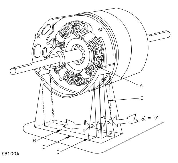
A – Motor winding to be shielded by barrier. This is to consist of the entire motor winding if it is not otherwise shielded, and is to consist of the unshielded portion of a motor winding which is partially shielded by the motor enclosure or equivalent.
