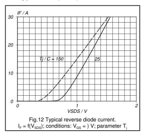
Because the diode operates as a bipolar device it is subject to charge storage effects. This charge must be removed for the diode to turn-off. The amount of charge stored is given by  $Q_{rr}$ , the reverse recovery charge, the time taken to extract the charge is given by  $t_{rr}$ , the reverse recovery time. NB. trr depends very much on the -dl/dt in the circuit,  $t_{rr}$  is specified in data at 100 A/µs.
