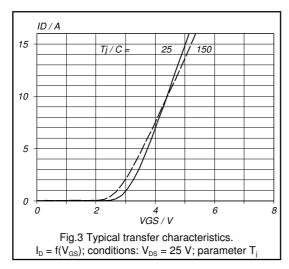
Useful plots in the graphical data are the typical transfer characteristics (Fig.3) showing drain current as a function of  $V_{\rm GS}$  and the gate threshold voltage variation with junction temperature (Fig.4). An additional plot also provided is the sub-threshold conduction, showing how the drain current varies with gate-source voltage below the threshold level (Fig.5).
