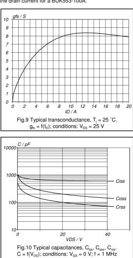
MOSFET refers to the flat portion of the output characteristics.) Fig.9 shows how  $g_{fs}$  varies as a function of the drain current for a BUK553-100A.
