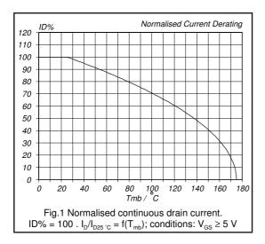
Obviously if the mounting base temperature was made equal to the max permitted junction temperature, then no power could be dissipated internally. A derating curve is given as part of the graphical data, an example is shown in Fig.2 for a device with a limiting  $T_i$  of 175 °C.
