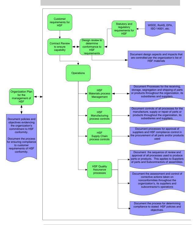
This model illustrates the minimum requirements of this standard, but does not show processes at a detailed level
