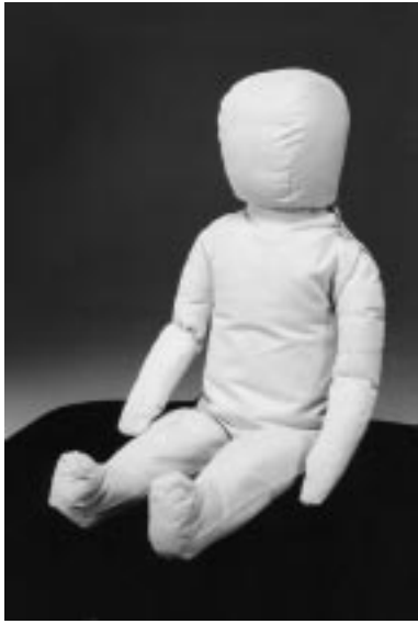
NOTE—This CAMI Infant Dummy was constructed in accordance with the Department of Transportation Specification dated April 29, 1975.
