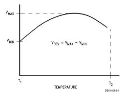
The average temperature coefficient of the reference input voltage,  ${\sim}V_{REF}$ , is defined as:
