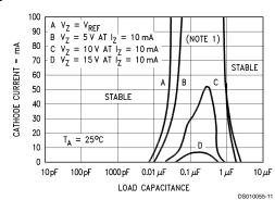
Note: The areas under the curves represent conditions that may cause the device to oscillate. For curves B, C, and D, R2 and V<sup>+</sup> were adjusted to establish the initial  $V_Z$  and  $I_Z$  conditions with  $C_L = 0$ . V<sup>+</sup> and  $C_L$  were then adjusted to determine the ranges of stability.
