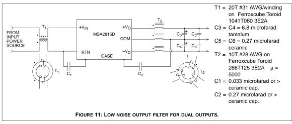
Balun net ampere turns are always zero, when used as in Figures 9 and 11, the only thing limiting small size is copper loss/temperature rise, the availability of small cores, and how physically small the balun can be made.
