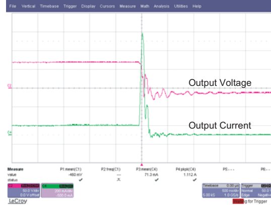
Fig. 6: Open Short Circuit Protection (500ns/div)
