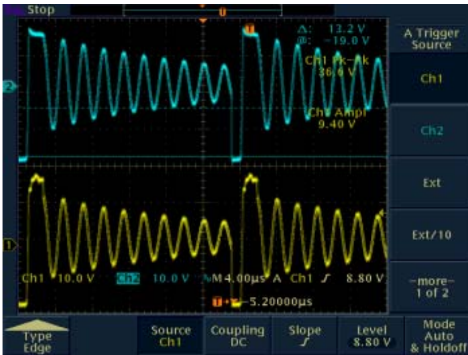
pic.3 secondary winding output and gate voltage of MOSFET waveform at no load condition .
