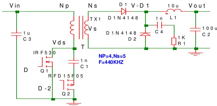
Purpose : This worksheet help to select the power components of forward series converter.
