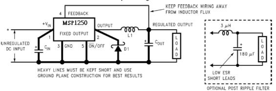
C<sub>IN</sub> --470  $~\mu$  F, 50V, Aluminum Electrolytic Nichicon "PL Series" C<sub>OUT</sub> --220  $~\mu$  F, 25V Aluminum Electrolytic, Nichicon "PL Series" D<sub>1</sub>--5A, 40V Schottky Rectifier, 1N5825 L<sub>1</sub> --68  $~\mu$  H, L38
