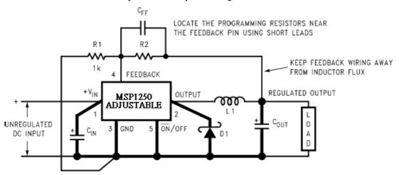
HEAVY LINES MUST BE KEPT SHORT AND USE GROUND PLANE CONSTRUCTION FOR BEST RESULTS
