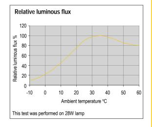
The fall-off rate of the luminous flux - i.e. the ratio of the luminous flux measured at 35°C and 25°C ambient temperature, respectively - may vary in the range between 1.05 and 1.25 depending on lamp type and electronic gear type used.
