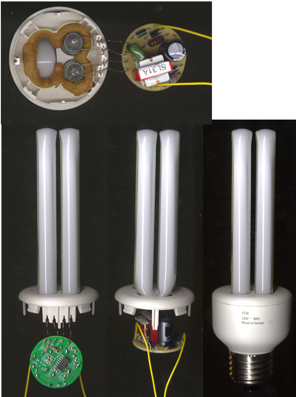
Figure 1: Photos of a 14W Compact Fluorescent Lamp with UBA2024T
