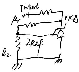
$$V_{KFF} = V_{ref} \left( 1 + \frac{P_1}{P_2} \right) + V_{ref} \times P_1$$
