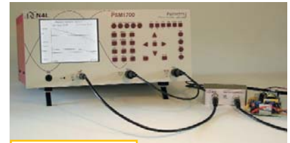
Figure 3 A typical test configuration for testing a switch-mode power supply has a phase-sensitive multimeter with two voltage-sensing measurement channels and a built-in signal generator that connects to the control loop via an injection transformer.
