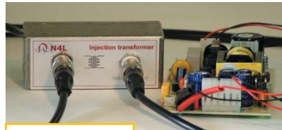
Figure 2 An injection transformer injects a disturbance signal into the control loop of an open-frame switched-mode power supply. At each injected frequency point, measure the relative amplitude in decibels and the relative phase in degrees.
