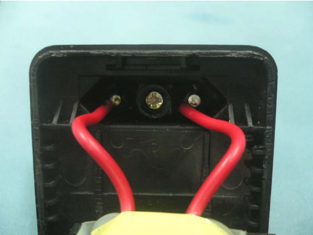
Fig. 4 Primary wire connection
