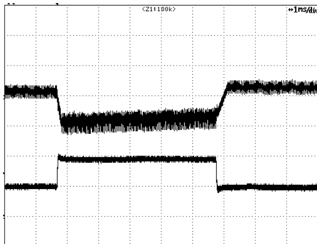
Figure 20 – Transient Response, 115 VAC, 50-100-50% Load Step. Upper: V_{OUT} 50 mV/div. Lower: I_{OUT} 0.5 A, 1 ms / div.
