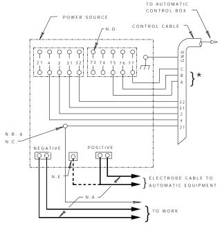
Above diagram shows electrode connected positive. To change polarity, turn power source off, reverse the electrode and work leads at the power source and position the switch on power source to proper polarity. Also reverse the leads on the back of the ammeter and voltmeter in the automatic control box.
