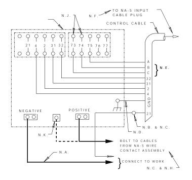
Above diagram shows electrode connected positive. To change polarity turn power off, reverse the electrode and work leads at the power source, position the positive - negative switch on the power source to correspond to the polarity of the electrode cable connection. Refer to NA-5 operating manual for required NA-5 control box polarity connections.
