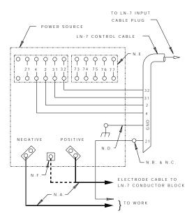
Above diagram shows electrode connected positive. To change polarity, turn power off, reverse the electrode and work leads at the power source and position the switch on power source to proper polarity.
