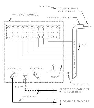
Above diagram shows electrode connected positive. To change polarity, turn power off, reverse the electrode and work leads at the power source, position the positive-negative switch on the power source to correspond to the polarity of the electrode cable connection. Refer to LN-9 operating manual for required polarity connections.
