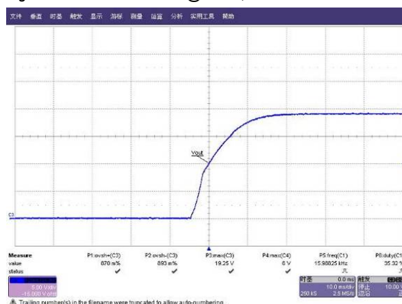
Fig. 8 Overshoot waveform @264Vac; no load
