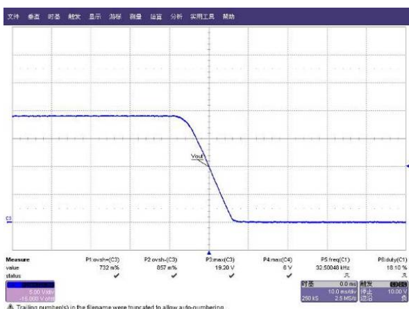
Fig. 9 Undershoot waveform @264Vac; full load
