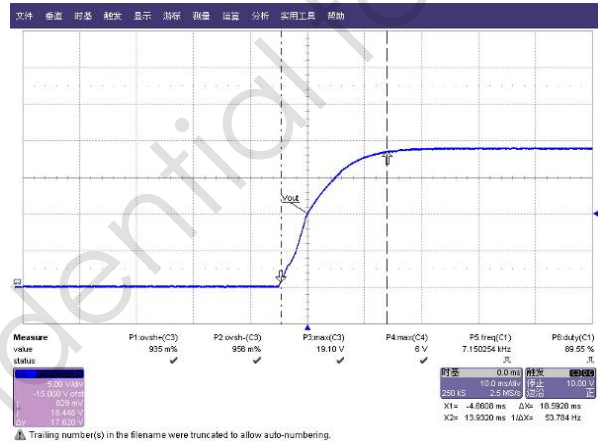
Fig. 19 Rise waveform @264Vac; full load
