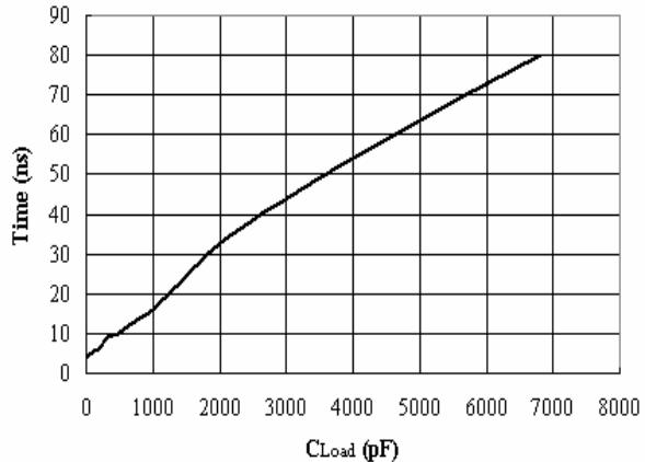
**Fihure 5 : Output Fall Time vs Load Capacitor**
