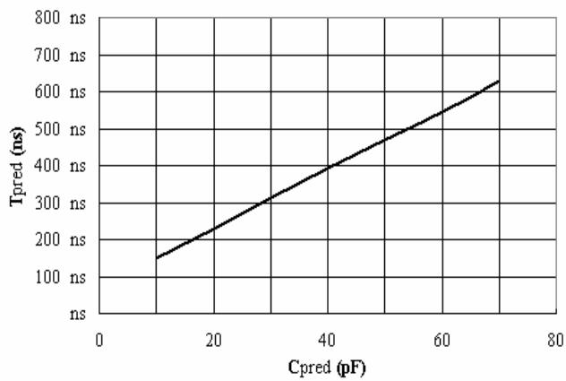
**Fihure 4 : Output Rise Time vs Load Capacitor**
