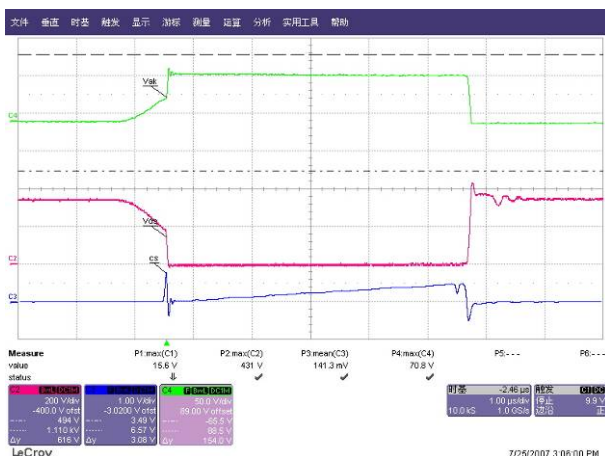
Fig. 29 Normal, Vds waveform@90 Vac/60Hz, full load
