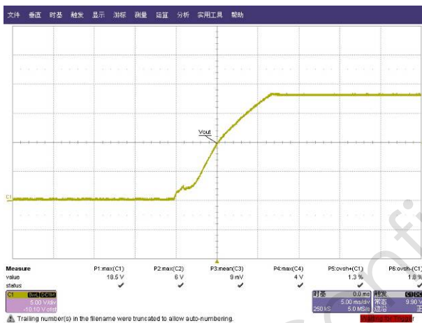
Fig. 9 Measured overshoot waveform@264Vac/50Hz, full load
