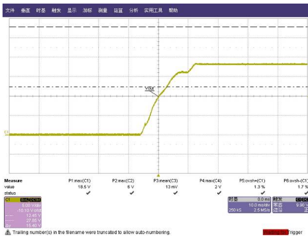
Fig. 7 Measured overshoot waveform@90Vac/60Hz, full load
