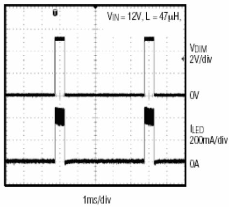
**PWM DIMMING AT 200Hz
