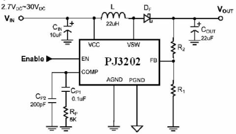
The PJ3202 develops a 1.276V reference from the FB pin to ground. Output voltage is set by connecting the FB pin to an output resistor divider and the maximum output voltage is determined by the VSW pin maximum voltage minus the output diode forward voltage. Referring to typical application circuit, the output voltage is set by the below formula(1):
