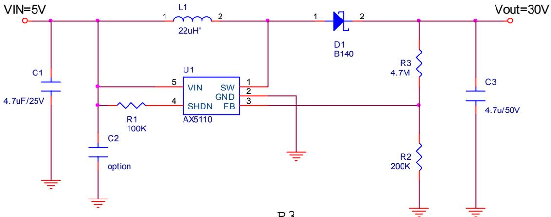
$$V_{out} = V_{FB} * (1 + \frac{R3}{R2})$$
