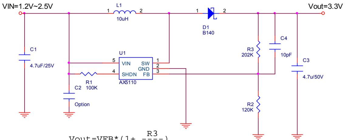
$$V_{out} = V_{FB} * (1 + \frac{R3}{R2})$$
