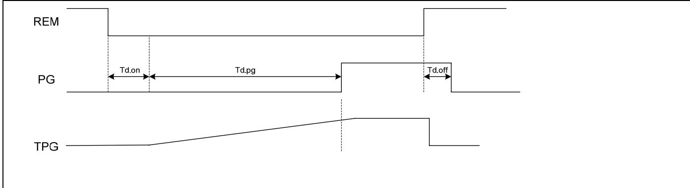
2. REM vs. Under Voltage Protection Delay time
