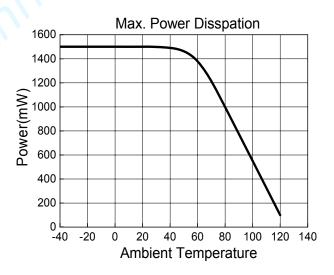
Note that the device power dissipation will most often be a maximum at minimum supply voltage. It will also increase if the efficiency of the circuit is low. This may result from the use of unsuitable coils, or excessive parasitic output capacitance on the switch output.
