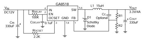
$R1=4.7K\Omega$ ,  $R2=1.5K\Omega$ ,  $T_{DELAY} = 1.147mS$
