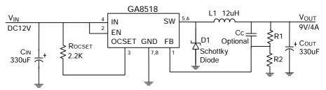
$V_{OUT} = V_{FB} x (1 + R1 / R2); R1=10.2K\Omega, R2=1K\Omega$
