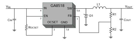
\*  $V_{OUT} = V_{FB} x (1 + R1/R2)$
