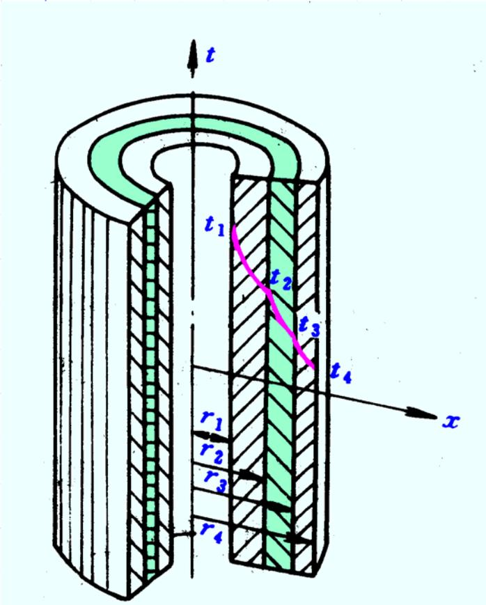
$$Q = \frac{2\pi L(t_1 - t_2)}{\frac{1}{\lambda_1} \ln \frac{r_2}{r_1}} = \frac{2\pi L(t_2 - t_3)}{\frac{1}{\lambda_2} \ln \frac{r_3}{r_2}} = \frac{2\pi L(t_3 - t_4)}{\frac{1}{\lambda_3} \ln \frac{r_4}{r_3}}$$
