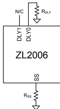
**Figure 14. DLY and SS Pin Resistor Connections**
