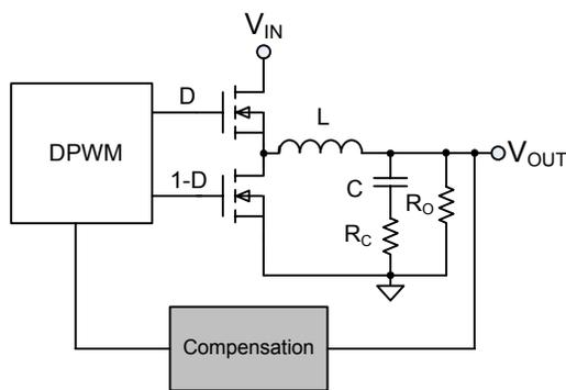
**Figure 18. Control Loop Block Diagram**
