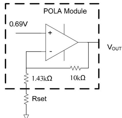
**Figure 11. Output Voltage Setting on POLA Module**
