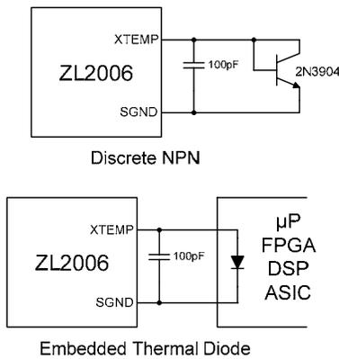
**Figure 21. External Temperature Monitoring**
