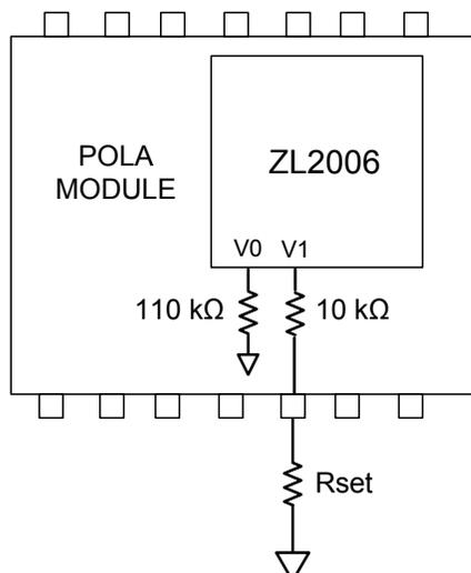
**Figure 12. R<sub>SET</sub> on a POLA Module**
