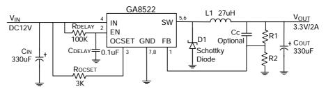
$R1=4.7K\Omega$ ,  $R2=1.5K\Omega$ ,  $T_{DELAY} = 1.147mS$
