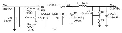
$R1=4.7K\Omega$ ,  $R2=1.5K\Omega$ ,  $T_{DELAY} = 1.147mS$
