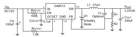
$R1=4.7K\Omega$ ,  $R2=1.5K\Omega$ ,  $T_{DELAY} = 1.147mS$
