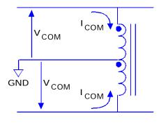
magnetic fields to be generated which cancel each other out. The effect is that the device presents zero impedance to common mode signals, shorting them directly to ground potential.
