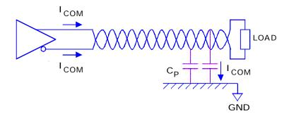
parasitic capacitance C<sub>P</sub>. In this case, the currents generate magnetic fields with equal magnitude and polarity, which do not cancel each other out. The common mode current is able to generate an electromagnetic field outside the spiral wound pair, which acts just like an antenna.
