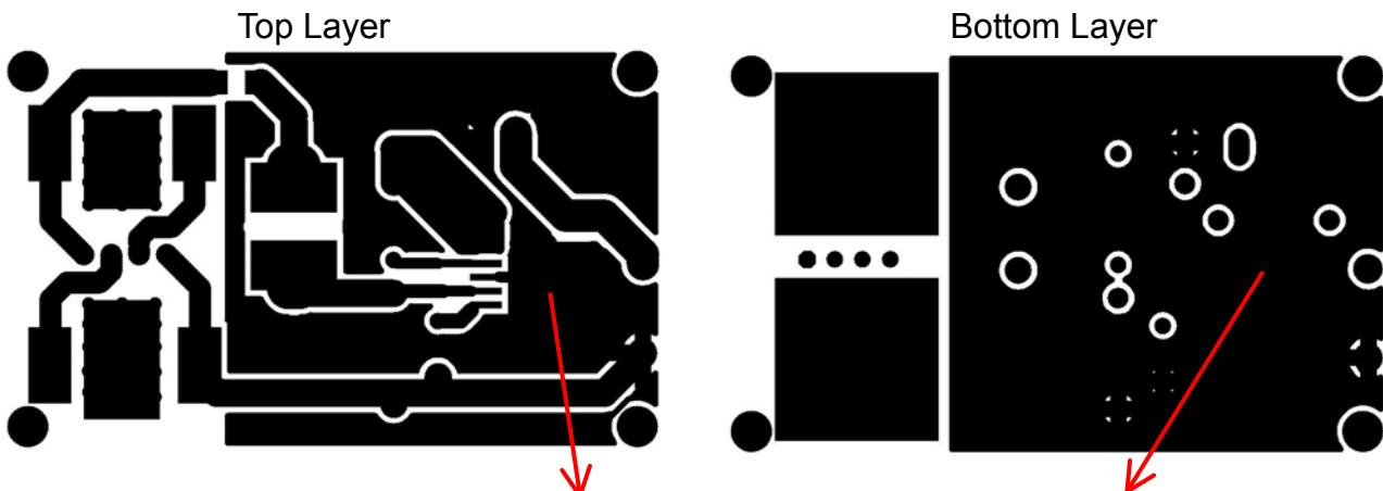
Large PCB area is reserved for GND plane and is connected to the heat pad of AMC7150.
