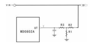
Voltage of UT for single Bat's voltage (about 2.1V), If charge many cell, must after according to R1 and R2 cent voltage receive UT(single cell's voltage). analysis as follows:
