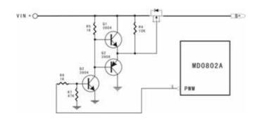
Bases current sampling's big and small and We needful current fixed value (50mV) that Comparative difference value and that ceaselessly tune up output pulse, thereby arrive at Pre-Charge, Fast Charge and Trickle Charge charged action.
