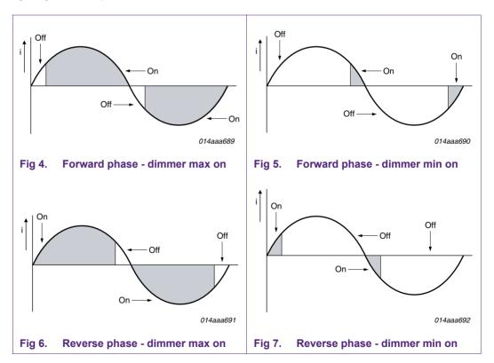
AN10754\_1 Application note Two switching methodologies can be distinguished: triac dimming and transistor dimming. Triac switching is always used with forward phase dimmers. Transistor switching can be used with forward and reverse phase dimmers. Transistor dimmers have the advantage of being able to switch capacitive loads, but most existing dimmers are still triac based.
