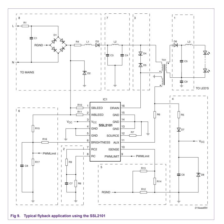
The mains voltage is rectified, buffered and filtered in the input section and connected to the primary winding of the transformer. The following functional blocks can be identified in the SSL2101 application (refer to Figure 9):
