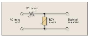
Coordinated overvoltage and overcurrent protection on an ac mains circuit is achieved with a circuit having one dedicated component for each event type.
