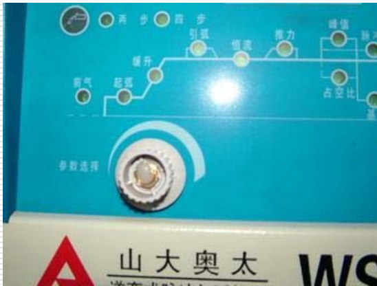
拆掉旋钮顶盖
