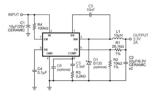
Figure 2 . MP1482 with 3.3V Output, 22µF/6.3V Ceramic Output Capacitor
