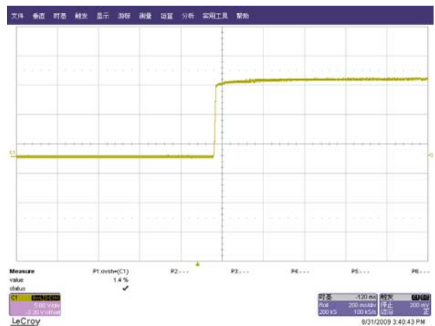
Fig. 8 Measured overshoot waveform@90Vac/60HZ, no load
