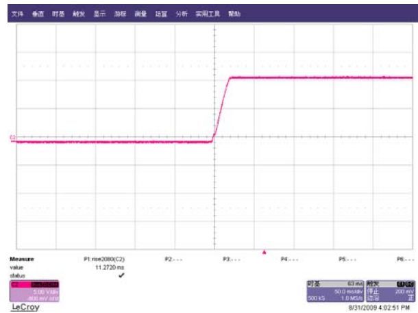
Fig. 16 Rise time measured waveform@100Vac/60HZ,full load
