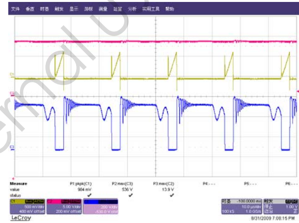
Fig. 25 Vdd, Sense & Vds waveform @264Vac/50Hz, full load
