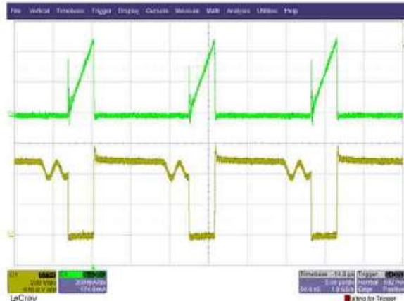
Figure 20 – 265 VAC, Full Load. Upper: I_{DRAIN} , 0.2 A / div. Lower: V_{DRAIN} , 200 V / div., 5 \mu s / div.
