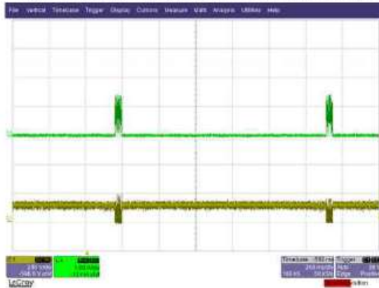
Figure 25 – 90 VAC, Full Load. Upper: I_{\text{OUTPUT}} , 1 A / div. Lower: V_{\text{DRAIN}} , 200 V, 200 ms / div.
