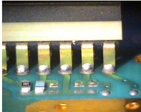
Figure 7 Good joints on board top side
