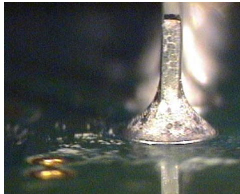
Figure 4 Good joint-board bottom side
