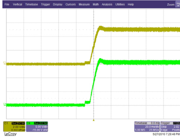
Figure 17 – Start-up Profile, 264 VAC. Upper: V_{5V} , 2 V / div. Lower: V_{16V} , 5 V, 20 ms / div.
