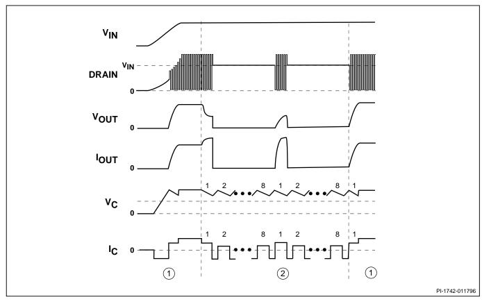
Figure 6. Typical Waveforms for (1) Normal Operation, (2) Auto-restart.
