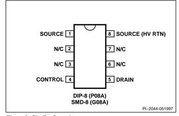
Figure 3. Pin Configuration.
