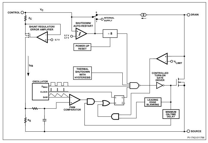
Figure 2. Functional Block Diagram.
