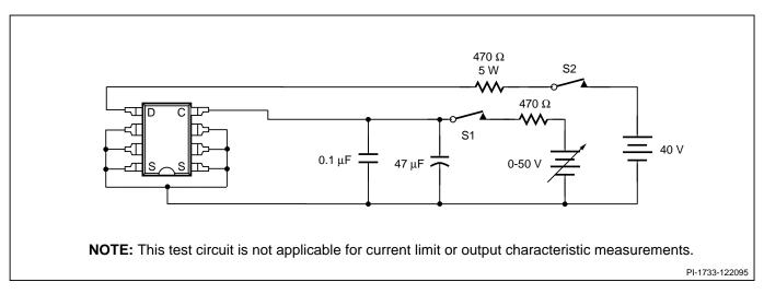
Figure 12. TOPSwitch General Test Circuit.
