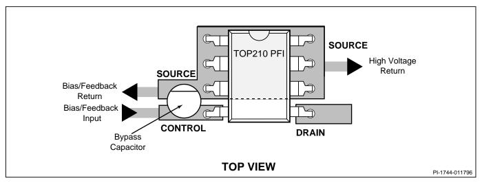
Figure 9. Recommended PC Layout for the TOP209/210.
