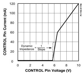
Figure 11. TOPSwitch CONTROL Pin I-V Characteristic.
