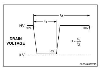
Figure 10. TOPSwitch Duty Cycle Measurement.
