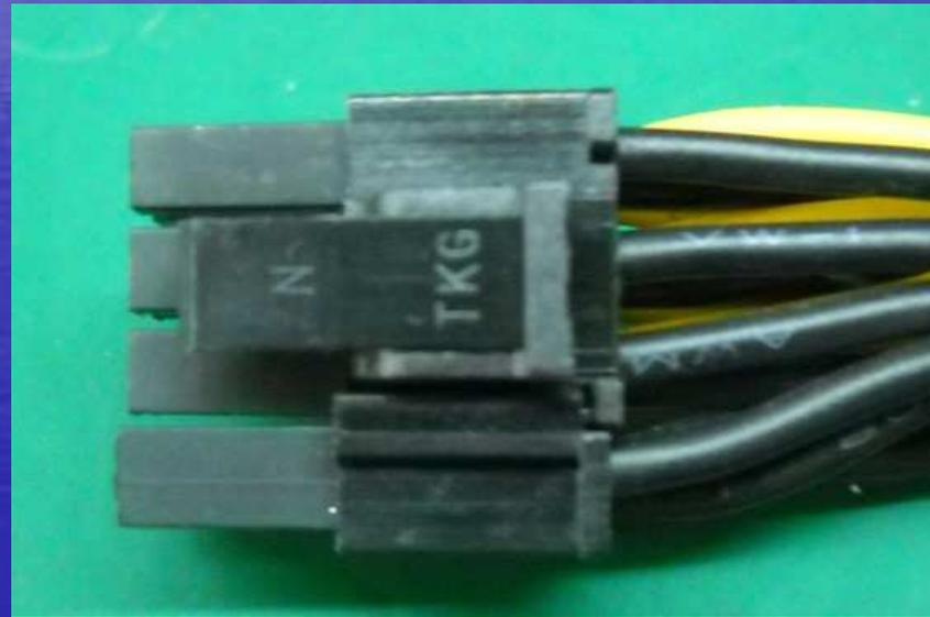
显卡6pin (3黄3黑) 6+2pin (组合8pin, 拆开就是6pin, 3黄5黑):
