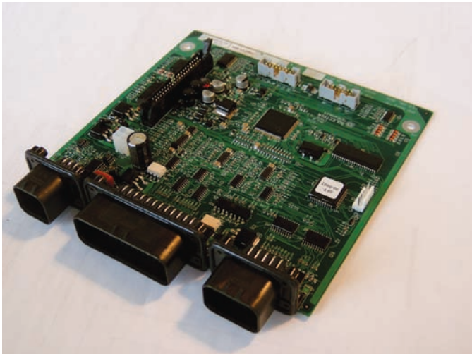
DSP control board Critical inverter functions rely on the software run on the DSP.
