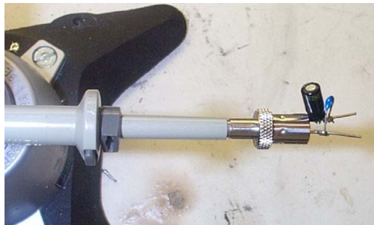
Figure 50 - Oscilloscope Probe with Probe Master ( www.probemaster.com ) 4987A BNC Adapter. (Modified with wires for ripple measurement, and two parallel decoupling capacitors added)
